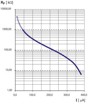
$$R_{F} = \frac{400 \, \mu A \, x \, 120 \, k\Omega}{I} - 120 \, k\Omega$$
